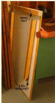
Folding leg brackets fasten the legs (see Source, right). A spring-loaded lever locks the legs open and closed.
